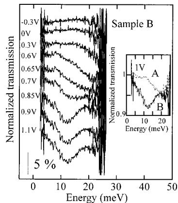
FIG. 3. Normalized far-infrared transmission of sample B as a function of the applied gate voltage. The curves have been offset for clarity. The inset shows a comparison between the normalized transmission of sample B (full line) and the transmission of sample A (dotted line) (1 V gate voltage).
