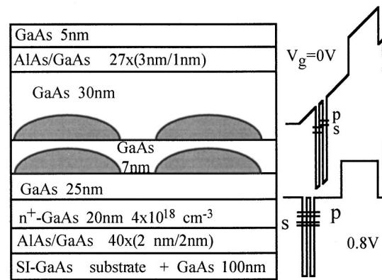
FIG. 1. Schematic structure of sample B. The inset shows the conduction band edge profile under two different applied gate voltages (0 and 0.8 V, respectively).
