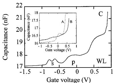
FIG. 2. Capacitance of sample C as a function of the applied gate voltage. The capacitance is measured at 4.2 K. The inset shows the capacitance of sample A (dashed line) and B (full line). The capacitance was measured at 34 Hz with a 5 mV tickle amplitude. The successive loading of *s,p*, and wetting layer states is indicated.
