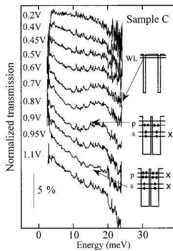
FIG. 4. Normalized far-infrared transmission of sample C as a function of the applied gate voltage. The curves have been offset for clarity. The inset explains schematically the spectra evolution.
