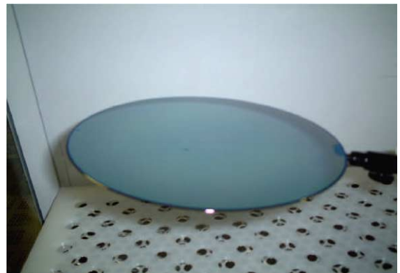
Fig. 10. A 200 mm relaxed SiGe on insulator substrate.
