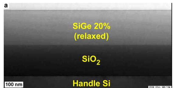
Fig. 11. Cross-sectional TEM image of a SiGe on insulator wafer (ready for strained Si epitaxial re-growth).
