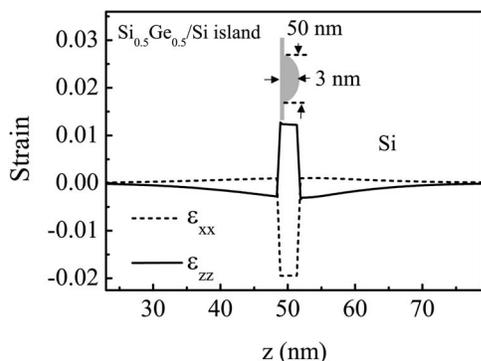
FIG. 5. Calculated strain components along the growth direction through the middle of a single island embedded in Si with 50% of Ge average composition. An island with a height of 3 nm and a base diameter of 50 nm is considered. The profile is obtained from a 3D finite-element calculation using a valence force field theory (Ref. 29).
