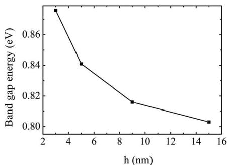
FIG. 8. Calculated interband recombination energy as a function of the island height for a 50% Ge composition. The line is a guide to the eye. A valence-band offset of  $0.47x$  is considered in the calculation.
