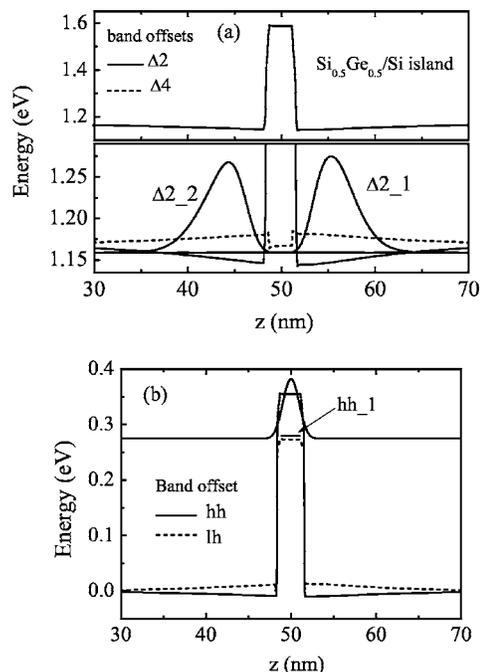
FIG. 6. (a) Band-edge alignment and confined states in the conduction band. A zoom of the conduction-band lineups is shown in the lower part of the figure. (b) Band-edge alignment in the valence band calculated using the 30-band  $\mathbf{k} \cdot \mathbf{p}$  model introducing strain profile of Fig. 5, i.e., for a single  $\text{Si}_{0.5}\text{Ge}_{0.5}$  island embedded in a silicon matrix. hh\_1 is the ground state energy level of the heavy hole.
