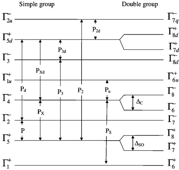
FIG. 1.  $O_h$  group bands involved in the 15-band  $\mathbf{k}\cdot\mathbf{p}$  model for simple group used by Cardona and Pollak (Ref. 15) and for double group used in the 30-band model at  $\mathbf{k}=\mathbf{0}$  (center of the Brillouin zone) in the Koster notation. (Ref. 31). The momentum matrix elements  $P_i$  which are used in the 30-band model are defined in Ref. 11.
