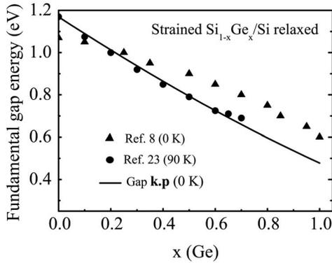
FIG. 2. Fundamental band-gap energy of strained  $\text{SiGe}/\text{Si}$  calculated within the framework of 30-band  $\mathbf{k}\cdot\mathbf{p}$  model (full line). The data reported in Ref. 8 (triangles) and in Ref. 23 (full dots) are given as comparison.
