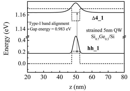
FIG. 4. Band lineup and resulting fundamental electron and hole confined levels and wave functions in strained  $\text{Si}_{0.7}\text{Ge}_{0.3}$ /Si quantum well with a 5 nm height, calculated within the framework of the 30-band model. The calculation uses an average valence-band offset given by Colombo *et al.* (Ref. 20). Note that the  $\Delta 4$  valley lineup (in the upper part of the figure) is not represented on the same scale as the hh valley lineup (in the lower part of the figure).
