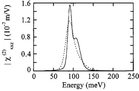
FIG. 6. Spectral dependence of the second-order nonlinear susceptibility  $|\chi_{xxz}^{(2)}|$  calculated in the valence band. Two distinct inhomogeneous broadenings are represented and correspond, respectively, to a 20% (dashed line) and a 10% (full line) dot size homogeneity.
