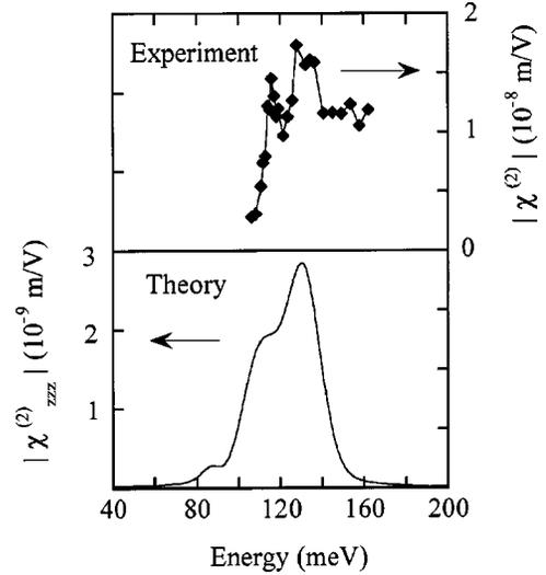
FIG. 8. Comparison between the susceptibility measured in TM polarization for  $p$ -type doped quantum dots and the second-order nonlinear susceptibility  $|\chi_{zzz}^{(2)}|$  calculated in the valence band (10% dot size homogeneity). Note the two different vertical scales.
