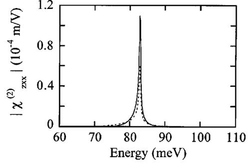
FIG. 3. Spectral dependence of the second-order nonlinear susceptibility  $|\chi_{zxx}^{(2)}|$  calculated in the conduction band. Two distinct inhomogeneous broadenings are represented and correspond respectively to a 20% (dashed line) and a 10% (full line) dot size homogeneity. The average quantum-dot height is 2.5 nm.
