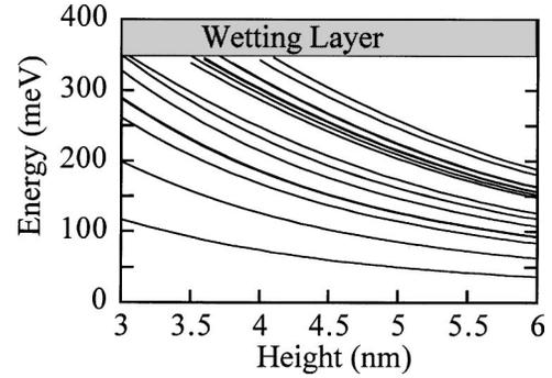
FIG. 2. Energy of the confined states in the valence band as a function of the quantum-dot height. The aspect ratio (height/diameter) is 0.2. The two-dimensional continuum wetting layer states are above 350 meV. Some states are not shown on the graph for quantum-dot heights larger than 5 nm.
