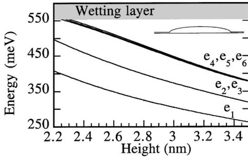
FIG. 1. Energy of the confined states in the conduction band as a function of the quantum-dot height. The aspect ratio (height/diameter) is kept constant and equal to 0.1. Above 560 meV, the confined states are hybridized with the wetting layer states. The two-dimensional wetting layer energy is found 40 meV below the GaAs conduction-band edge. The inset shows the quantum-dot geometry. Only the first six states are represented and some states are omitted for quantum-dot height larger than 3 nm.
