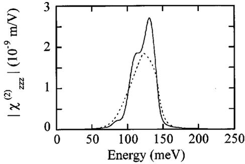
FIG. 4. Spectral dependence of the second-order nonlinear susceptibility  $|\chi_{zzz}^{(2)}|$  calculated in the valence band. Two distinct inhomogeneous broadenings are represented and correspond, respectively, to a 20% (dashed line) and a 10% (full line) dot size homogeneity.
