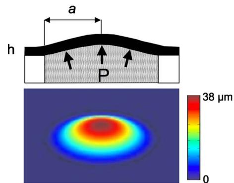
FIG. 1. (Color online) Top: schematic view of the bulge test. The radius  $a$  of the membrane and the thickness  $h$  of the sample are indicated. The liquid is illustrated by the gray area. Bottom: calculated deformed shape of a 28  $\mu\text{m}$  thick germanium membrane strained by a 2.5 MPa load pressure. The vertical scale varies from 0 to 38  $\mu\text{m}$ . The diameter of the blister is 1.45 mm.
