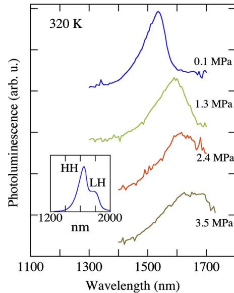
FIG. 3. (Color online) Room temperature PL spectra of the germanium membrane for different load pressures indicated on the right hand side of the figure. The curves have been offset for clarity. The inset shows the calculated recombination spectrum under a 0.7% strain, highlighting the contribution of heavy holes and light holes. The signal-to-noise ratio is smaller at large load pressures because of the detector cutoff.
