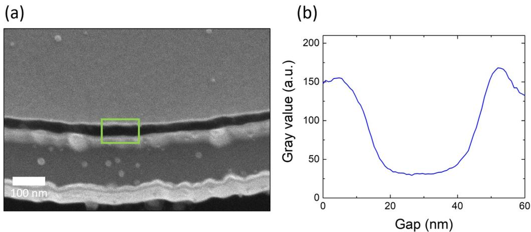
**Figure S1.** (a) SEM image of a nominally 50 nm gap and (b) gray scale profile along the vertical direction and integrated along the horizontal direction of the rectangle in (a), giving a gap of 45 nm at the top.
