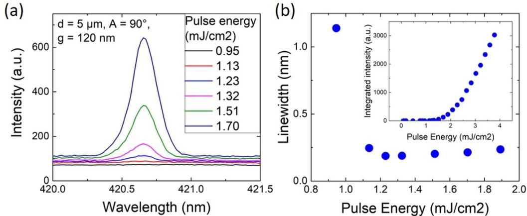
**Figure S7.** (a) Pulse-energy dependent spectra around threshold for a device with  $A = 90^\circ$  and  $g = 120$  nm. The threshold is at 1.2 mJ/cm<sup>2</sup> per pulse. (b) Linewidth vs. pulse energy of the mode in (a) and (inset) integrated intensity vs. pulse energy for the same mode.
