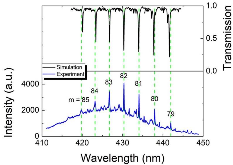
**Figure S2.** Simulated (top) and experimental (bottom) spectra of a device with  $A = 90^\circ$  and  $g = 50$  nm (simulated) and 45 nm (experimental). The azimuthal orders of the first-order radial modes are  $m = 85$  to 79.
