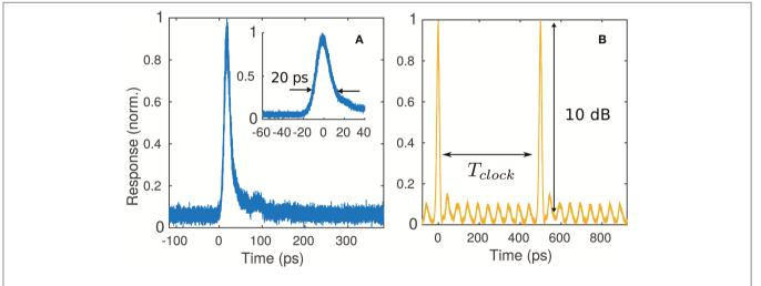
**FIGURE 9** | Characterization of the gate function, for an CW input signal **(A)** and a signal modulated at 20 GHz **(B)**. The sampling rate is 2 GS/s, corresponding to the visible 500-ps period in **(B)**. The acquisitions are taken and averaged by a 70 GHz sampling oscilloscope. We observe an increase in transmission at each pulse clock: the gate is opened with a 10 dB contrast and a switching window of 20 ps taking into account the response of the photodiode.
