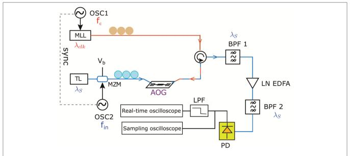
FIGURE 8 | Experimental set-up for all-optical sampling experiment. MLL, mode-locked laser; TL, tunable laser; OSC, RF synthesizer; MZM, Mach-Zehnder modulator; AOG, all-optical gate; BPF, bandpass filter; LN EDFA, low-noise EDFA; PD, photodiode; LPF, lowpass filter. The optical paths of the clock (c/k) and the signal (s) are colored in red and blue, respectively.
