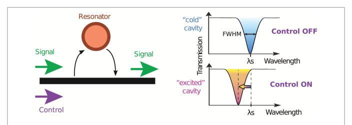
FIGURE 1 | Working principle of an AOG based on a resonator. (Left) Side-coupled configuration, the resonator is located next to the waveguide carrying the signal to be processed and the control signal. (Right) A control pulse induces a non-linear effect in the resonator, thereby modulating the signal transmission. FWHM, full width at half maximum.
