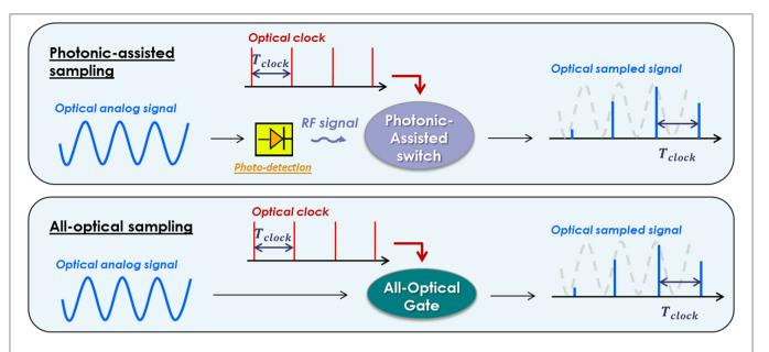
FIGURE 7 | Comparison between photonic-assisted and all-optical sampling. Photonic-assisted switches require an RF analog input, implying optical-to-electrical conversion of the incoming optical analog signal. In contrast, all-optical sampling devices can directly process optical signals, avoiding electrical conversion. In both configurations, at the output of the sampling device one retrieves the clock pulses modulated by the amplitude of the input analog signal.
