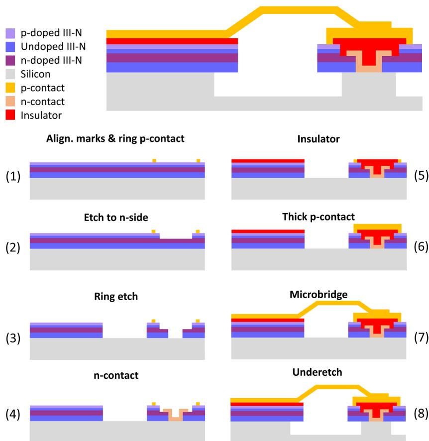
Fig. 1. Process flow of microrings for electrical injection.
