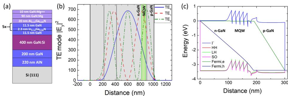
Fig. 3. The sample structure: a) Detailed heterostructure, b) Simulated mode confinement of the  $\text{TE}_0$ ,  $\text{TE}_1$ , and  $\text{TE}_2$  modes, the MQW region is highlighted in green, the heterostructure in gray, c) Energy band structure of the sample at 3.4 V bias.
