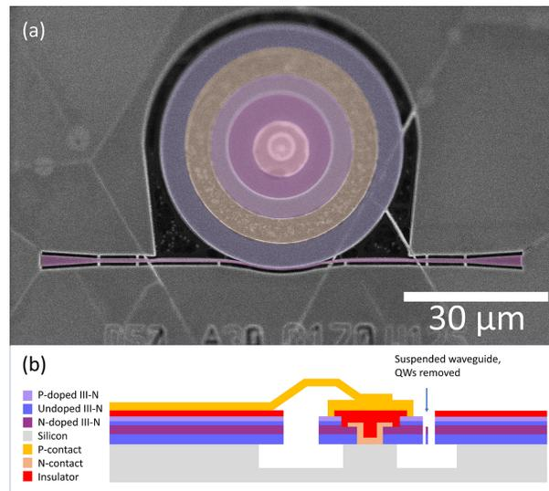
Fig. 6. Microring under electrical injection with bus waveguide side coupling: a) False color SEM image of device with a  $50\ \mu\text{m}$  diameter ring and a  $100\ \mu\text{m}$  long bus waveguide after several processing steps. b) Side-view sketch of a full device.
