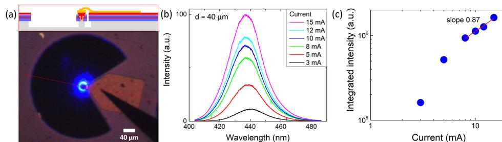
Fig. 5. Measurement results: a) Top: Cross-sectional view of the device along the red dashed line. Bottom: Photo of a powered 40  $\mu\text{m}$  diameter device emitting blue electroluminescence. b) Spectra of a device with a 40  $\mu\text{m}$  diameter at different injection currents. Maximum current density 4.2  $\text{kA}/\text{cm}^2$ . c) Integrated intensity of the measurements in b).
