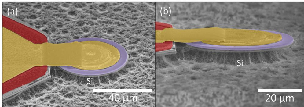
Fig. 2. a) False color SEM images of a 50  $\mu\text{m}$  diameter microring for electrical injection. b) Same device but from a different angle to emphasize the underetching of the microring. The metal microbridge and p-contact are highlighted in yellow, the insulator in red, and the III-nitride in purple. The rough gray area is the etched silicon.
