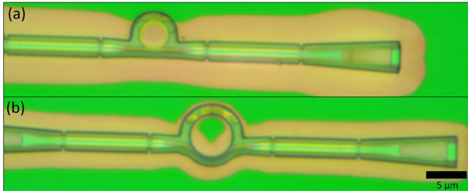
Figure S9: Optical microscope images of a) a  $3\ \mu\text{m}$  diameter disk with a straight waveguide and b) a  $5\ \mu\text{m}$  diameter disk with a  $90^\circ$  bent waveguide. The underetch and silicon pedestal are visible.
