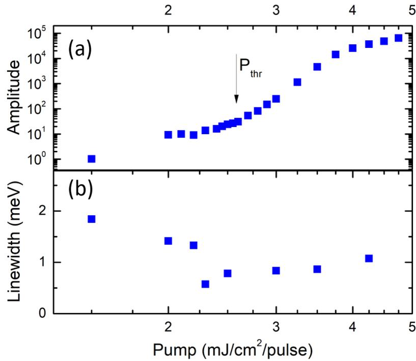
Figure S7: Pump energy-dependent measurement of a 4  $\mu\text{m}$  diameter microdisk laser without a waveguide fabricated on the same wafer, showing a) amplitude and b) linewidth of the lasing mode at 416.5 nm.
