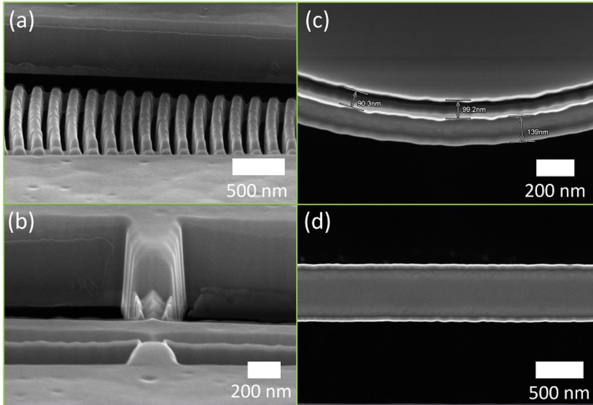
Figure S10: Close-up SEM images of various parts of the photonic circuit. a) Side-view of a grating coupler at a  $20^\circ$  angle. b) Side-view of a tether and waveguide at a  $20^\circ$  angle. c) Top-view of a disk and waveguide depicting a gap of 90 - 100 nm. d) Top-view of the wide part of a waveguide.
