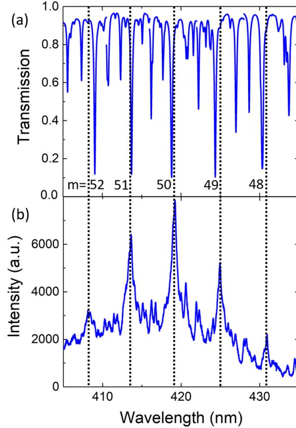
Figure S2: Comparison of a) simulation and b) measurement for a 3  $\mu\text{m}$  diameter disk. The mode positions match well and the azimuthal numbers of the first order radial modes is clearly identified.
