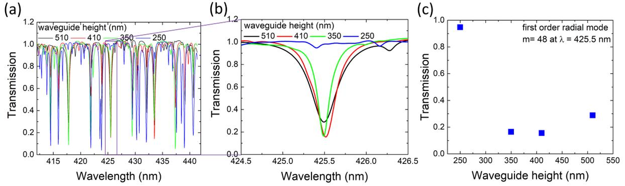
Figure S4: FDTD simulation of the influence of the waveguide height on the coupling strength. a) Transmission over a 30 nm wavelength range for a waveguide height between 250 nm and 510 nm. b) Zoom-in on the first-order radial mode with azimuthal order  $m = 48$  at 425.5 nm. c) Transmission over waveguide height for the same mode as in b).
