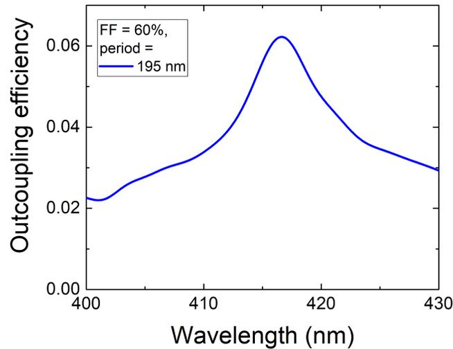
Figure S5: FDTD simulation of an out-coupling grating with a 195 nm period and a fill-factor of 60%, giving an outcoupling efficiency of 6% at 417 nm.
