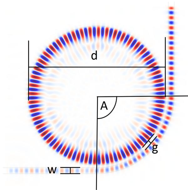
Figure S1: Simulation of the  $H_z$  field of a  $d = 3 \mu\text{m}$  diameter disk for a first order radial mode with azimuthal order  $m = 48$ . The waveguide is bent at a  $A = 90^\circ$  angle, the gap is  $g = 50$  nm and the waveguide width is  $w = 133$  nm.
