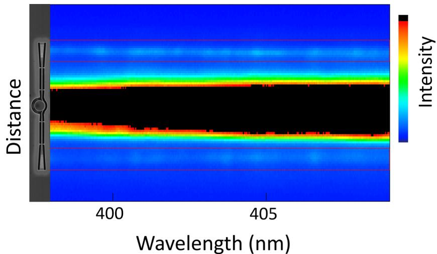
Figure S8: Over-saturated intensity map of the CCD with corresponding SEM image of a device on the left side. Same image as figure 2 a) in the manuscript, but with a different color scale to highlight the emission at the gratings. The gratings are indicated in red.
