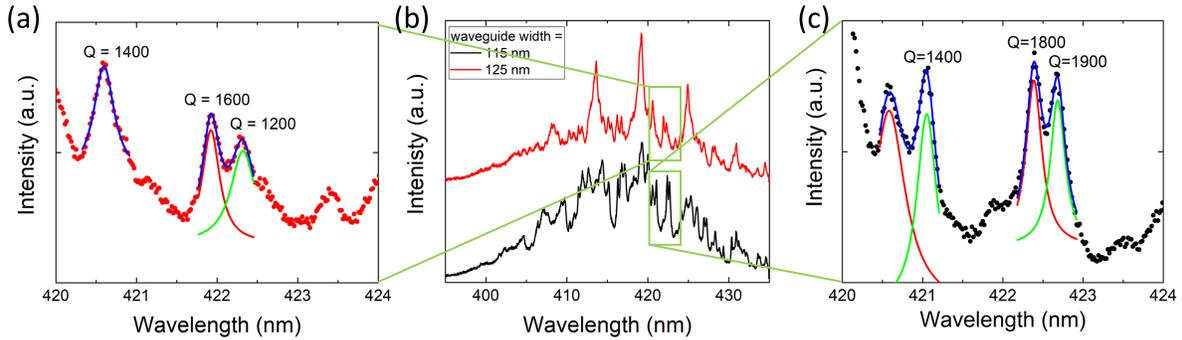
Figure S6: Loaded Q factor of two devices with a disk diameter of  $3\ \mu\text{m}$ , a waveguide bending angle of  $90^\circ$ , a gap of  $90\ \text{nm}$ , and waveguide widths of  $115$  to  $125\ \text{nm}$ . a) Zoom-in of the  $w = 125\ \text{nm}$  curve and Lorentzian fits giving loaded Q factors of  $1200$  to  $1600$ . b) Full spectra of both devices. c) Zoom-in of the  $w = 115\ \text{nm}$  curve and Lorentzian fits giving loaded Q factors of  $1400$  to  $1900$ .
