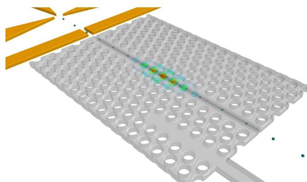
*Principle diagram of what could be an on-chip non classical light source. Electrons from the electron gun (yellow, composed of cathode, grid and anode) move across a slotted photonic crystal (PhC – in grey on the picture, 10- $\mu$ m long here). While traveling through the PhC, they excite the optical mode in the center of the PhC. The light can be extracted thanks to the guide coupled to the cavity (bottom).*
