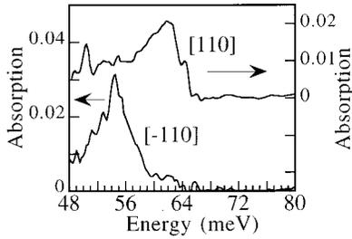
FIG. 1. Room-temperature absorption of the  $n$ -doped quantum dot sample. The absorption is measured at normal incidence. The transmission is normalized by the transmission of an undoped GaAs substrate with an identical thickness. The absorption is polarized along the  $[100]$  and  $[-110]$  directions.
