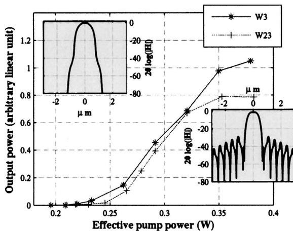
FIG. 3. Light-light characteristics of W3 and W2/3 lasers with PhC periods of 500 and 440 nm, respectively. Top inset:  $H$ -field profile of the fundamental W3 waveguide mode calculated for  $a/\lambda=0.316$  (wave vector  $k=0$ ). Bottom inset:  $H$ -field profile of the fundamental W2/3 waveguide mode calculated for  $a/\lambda=0.276$  [wave vector  $k=\pi/(a\sqrt{3})$ ].
