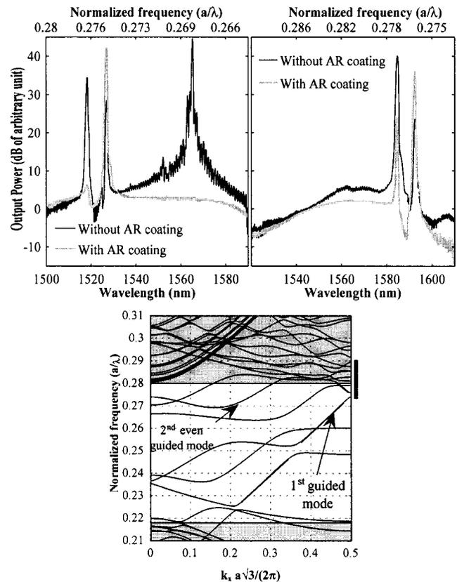
FIG. 2. Top panel: measured spectra of W2/3 lasers with and without AR coating (gray and black curves, respectively). Top left: lattice period of 420 nm. Top right: lattice period of 440 nm. Bottom panel: W2/3 waveguide band diagram ( $\Gamma M$  direction) with the gain region indicated on the right for a PhC period of 440 nm.
