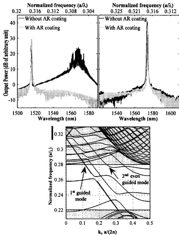
FIG. 1. Top panel: measured spectra of W3 lasers with and without AR coating (gray and black curves, respectively). Top left: lattice period of 480 nm. Top right: lattice period of 500 nm. Bottom panel: W3 waveguide band diagram ( $\Gamma K$  direction) with the gain region indicated on the left for a PhC period of 500 nm.
