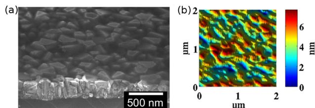
FIG. 1. (a) SEM view of a rough polycrystalline diamond layer covered by a flat silica layer during the smoothing process. (b) Atomic force microscope (AFM) image of the fully smoothed polycrystalline diamond. The measured RMS roughness is 1.6 nm.
