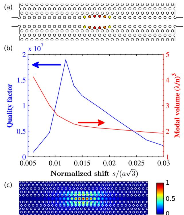
FIG. 3. Structure and simulations. (a) Structure of the cavity: the holes in warm colors define the cavity. For clarity, the shifts have been exaggerated. The red, orange, and yellow holes are shifted by a distance  $s$ ,  $2s/3$ , and  $s/3$ , respectively. (b) Simulated quality factor and modal volume of the cavities as a function of the normalized shift. (c) Module of the electric field component perpendicular to the waveguide axis (arbitrary unit).
