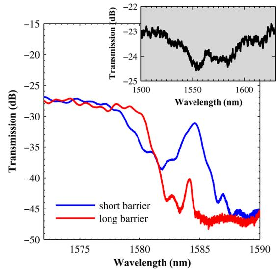
FIG. 4. Transmission spectra of the photonic crystal cavities for two barrier lengths. Inset: transmission spectrum of a single suspended ridge waveguide with its tapers.
