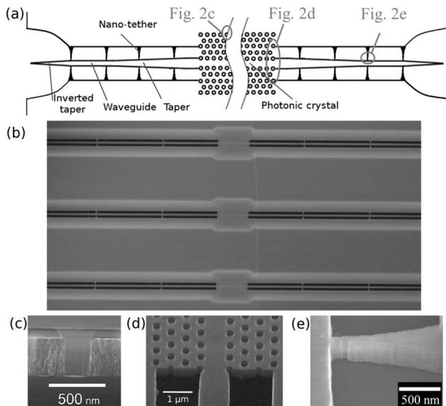
FIG. 2. Fabricated structures. (a) Schematic view of the fabricated structure. (b) SEM view of three photonic crystal cavities with their access waveguides suspended by nanotethers. (c) Cross section of an etched hole in nanocrystalline diamond layer before the removal of the silica mask. (d) Tilted view ( $45^\circ$ ) of a PhC and its access waveguide. (e) Tilted closed view of the access waveguide and a nanotether, the width of which is 70 nm at the side supporting the waveguide.
