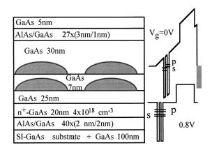
FIG. 1. Schematic structure of sample B. The inset shows the conduction band edge profile under two different applied gate voltages (0 and 0.8 V, respectively).
